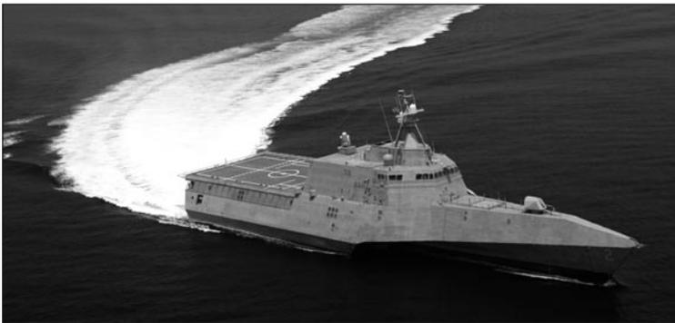
The General Dynamics design is a trimaran with a slender stabilized monohull. The sea frame is based on an Austal design for a fast car and passenger ferry.
