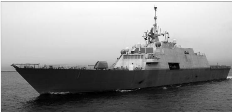
The Lockheed Martin design is a high speed semi-planing monohull based on a Ficantieri designed commercial vessel.
